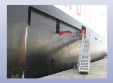
Accommodation ladder fully made of aluminumaccording to standard ISO 5488:1979.
